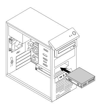
Figure 23. Installing the card reader
